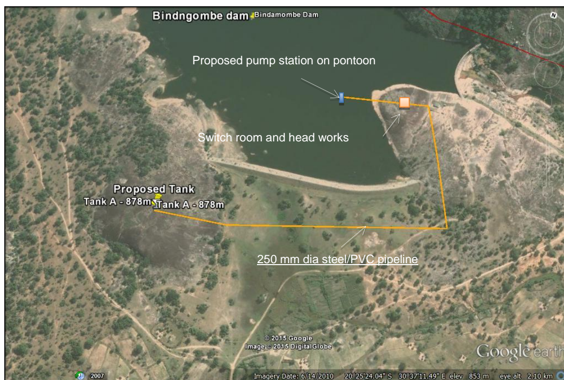
Figure 7 Location of proposed intake and pump station on pontoon
