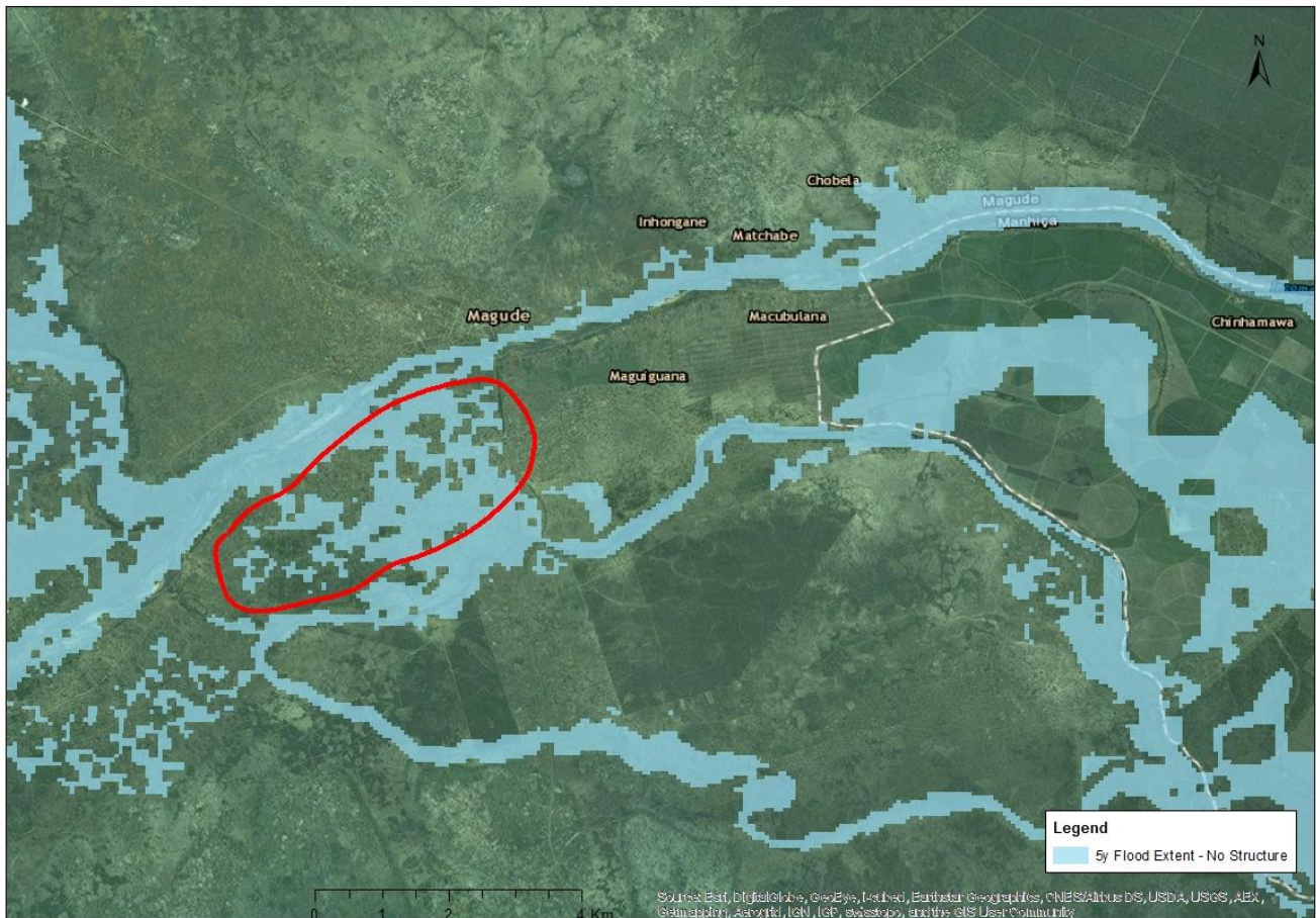
Figure 7-21 Maximum 1 in 5 Year Flood Extent for the S4F scenario and location of embankment failure.
